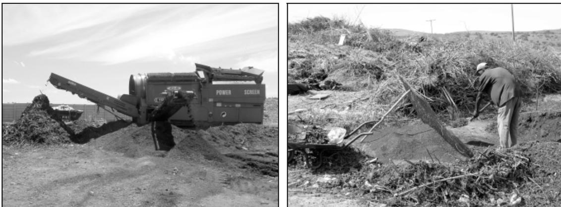
*Figure 13 Examples of sifting, done mechanically in a large scale project and manually in a small scale project*
