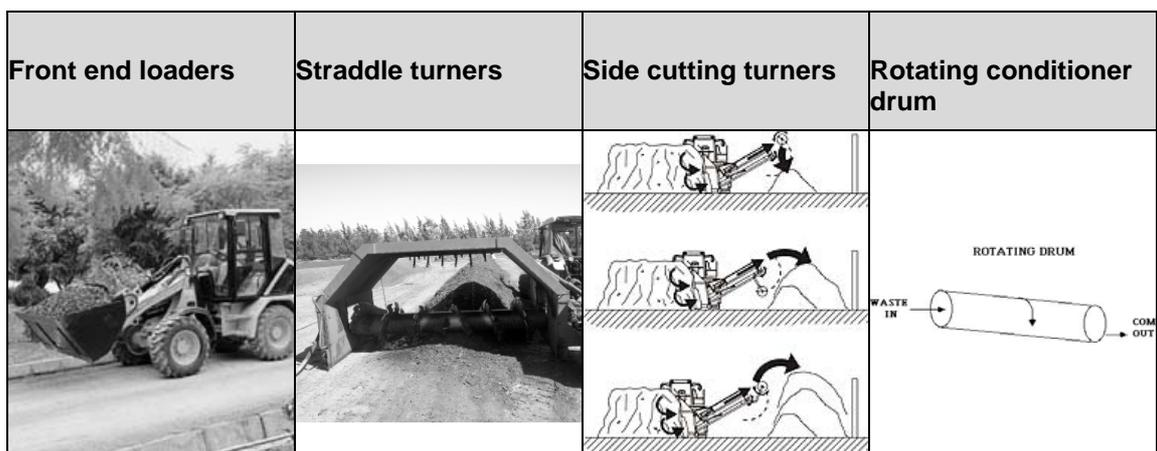
Figure 3 Examples of different machines for turning compost
