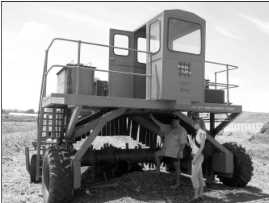
*Figure 8 Pikitup selfpowered straddle turner manufactured in South Africa*
