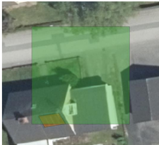
Figure 6b: Ch t ¾f suggested area with a ST system (green square) and identified ST system (orange polygon).
