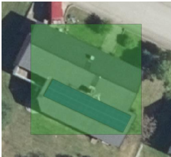
Figure 6a: Afrödullø suggested area with a PV system (green square) and identified PV system (blue polygon).
