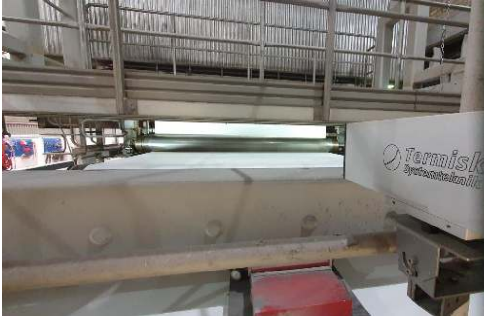
Figure 3 The location of the IR-camera (labelled Termisk Systemtechnik) aimed at the paperboard web (the white area in the middle of the picture)
