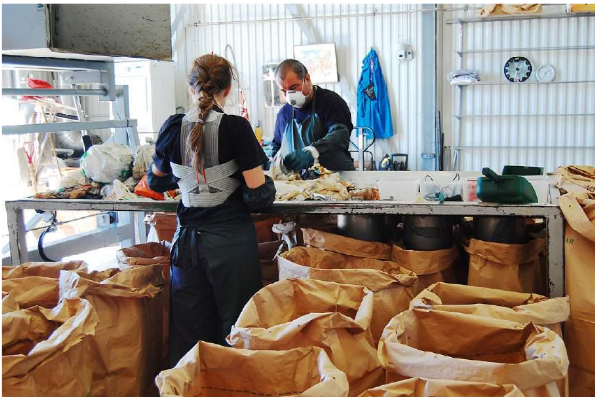
Figure 2: Sorting the waste into material components by hand during a conduction of a picking analysis (Vukicevic, 2016)
