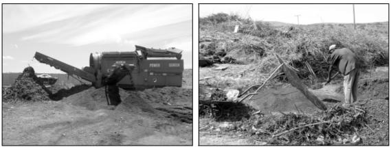
*Figure 13 Examples of sifting, done mechanically in a large scale project and manually in a small scale project*
